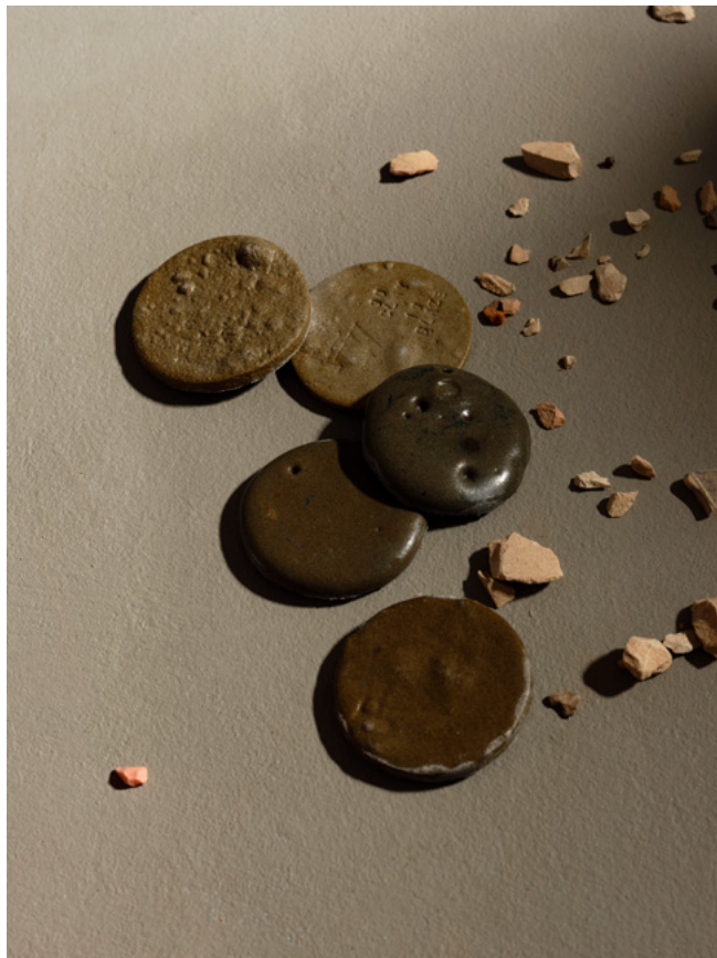
A collection of test tiles, blending a mixture of glaze waste and clay waste in increments of 10%, up to 50%.
