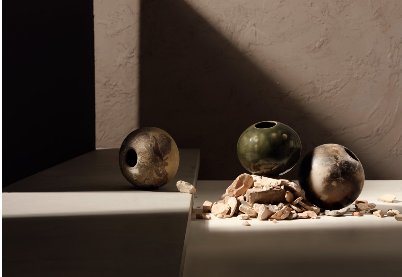
Collection of tests, left to right: Micro waste clay blend, waste glaze blend, smoke fired surface.
