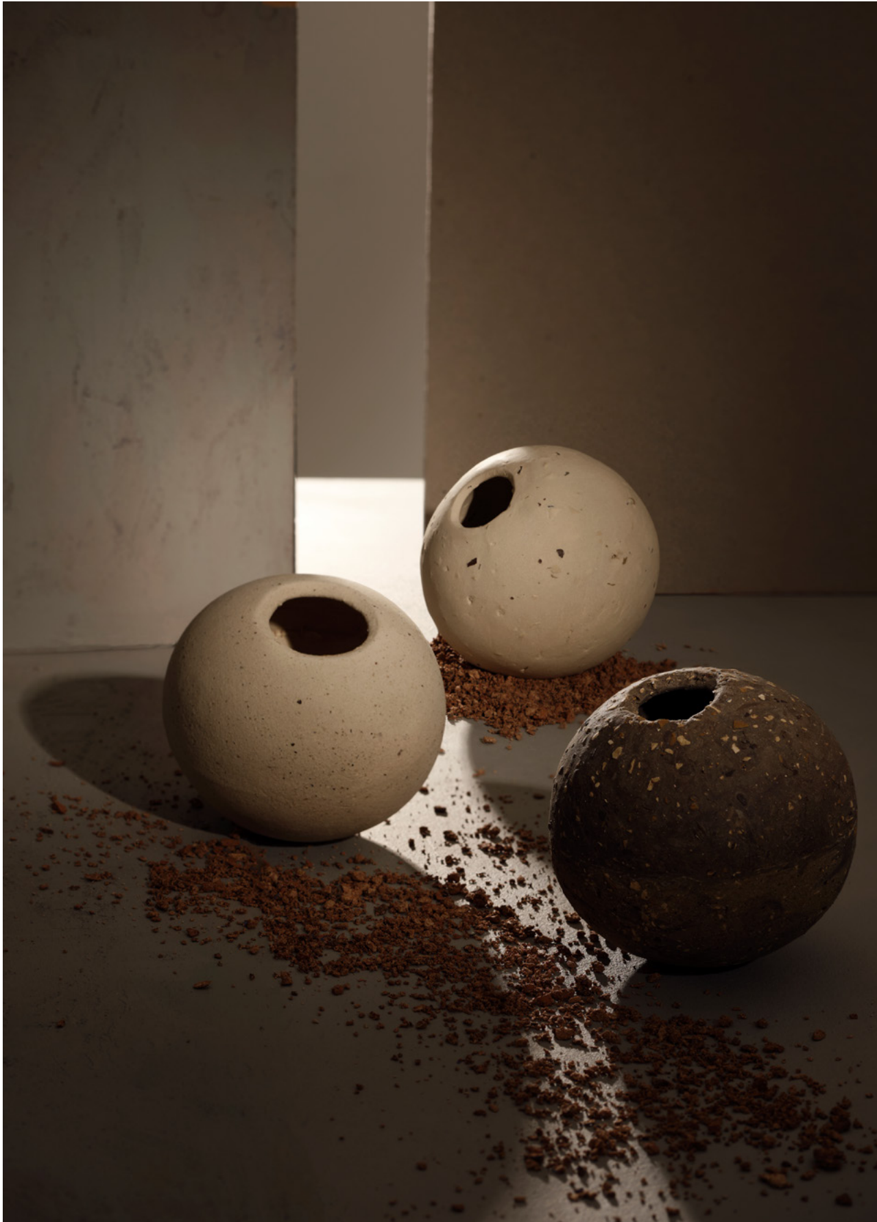
Grog tests, blending fired bisque waste at 5% or 10% with clay body.
