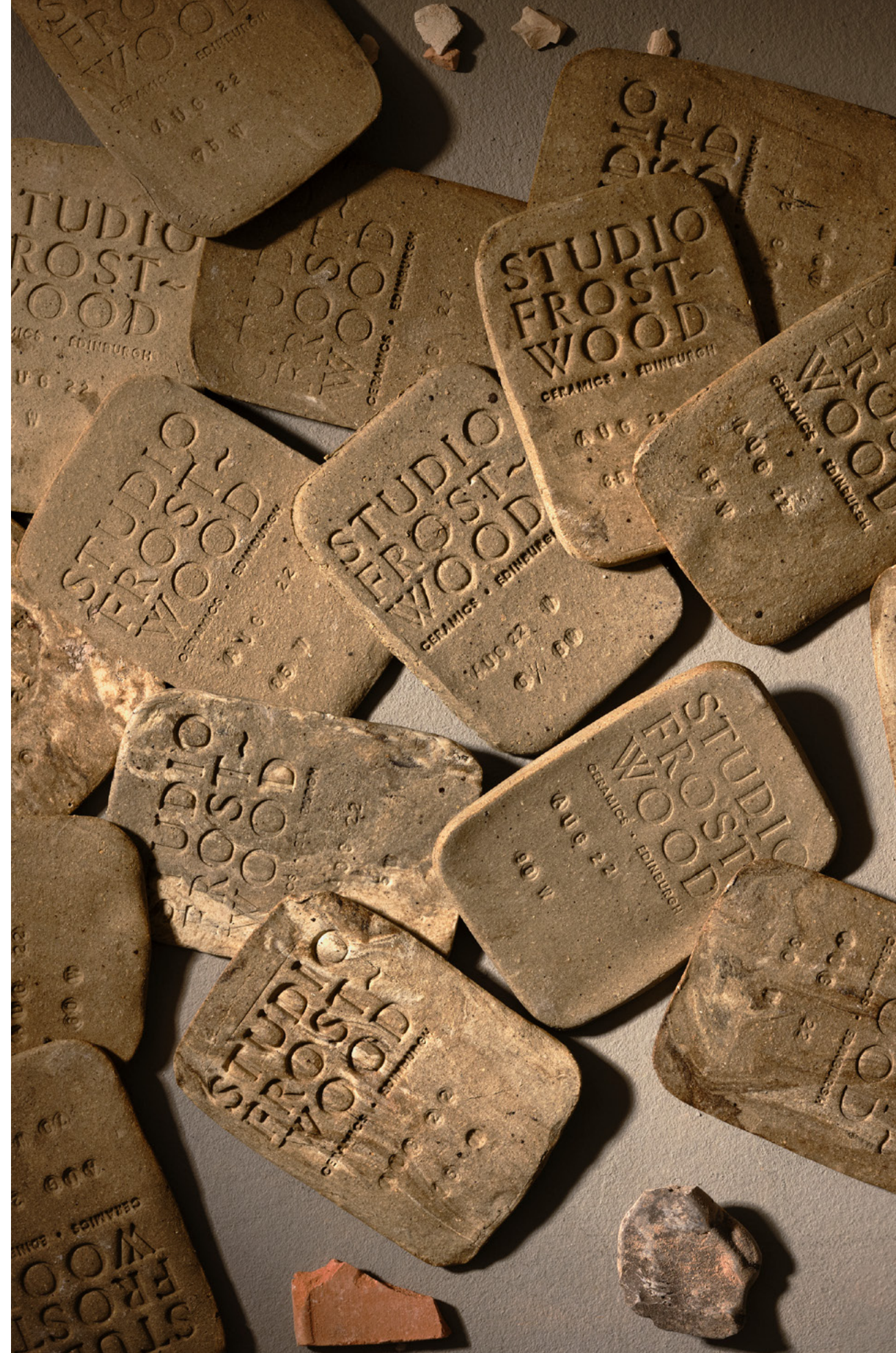
Test tiles, representing the blending of clay through wedging.
